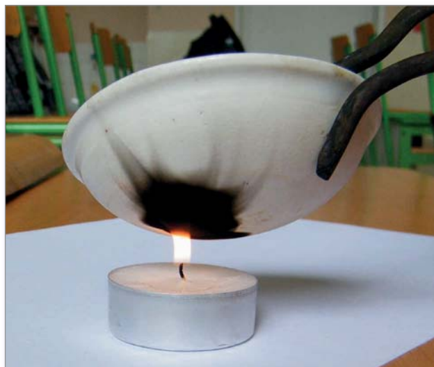
Figure 2. Chemical evidence for the presence of carbon in paraffin by formation of soot
