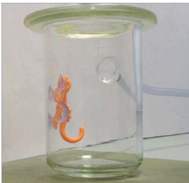
Figure 1. Suction cup Gecko under vacuum.
