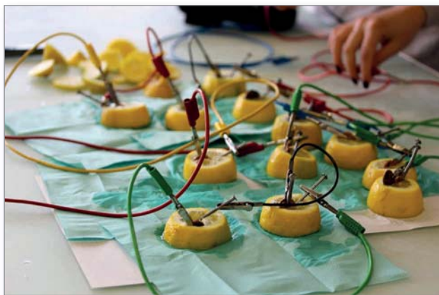
Figure 1. Battery that makes a light emitting diode glow
